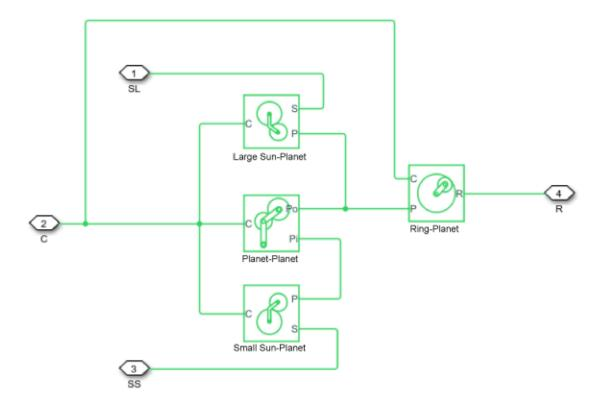
To increase the fidelity of the gear model, you can specify properties such as gear inertia, meshing losses, and viscous losses. By default, gear inertia and viscous losses are assumed to be negligible. The block enables you to specify the inertias of the internal planet gears. To model the inertias of the carrier, large sun, small sun, and ring gears, connect Simscape Inertia blocks to ports  $\mathbf{C}$ ,  $\mathbf{SL}$ ,  $\mathbf{SS}$ , and  $\mathbf{R}$ .
