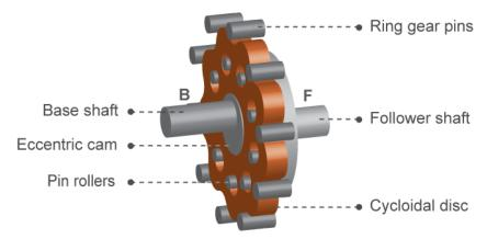
During normal operation, the base shaft drives the eccentric cam. The cam spins inside the cycloidal disc, causing it to rotate in an eccentric pattern about an offset axis. As it moves, the cycloidal disc engages the internal teeth of the ring-gear housing. The internal meshing reverses the rotational velocity direction.
