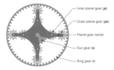
Structurally, the double-pinion planetary gear resembles a Ravigneaux gear without its second, large, sun gear. The inner planet gears mesh with the sun gear and the outer planet gears mesh with the ring gear. Because it contains two planet gear sets, the double-pinion planetary gear reverses the relative rotation directions of the ring and sun gears.
