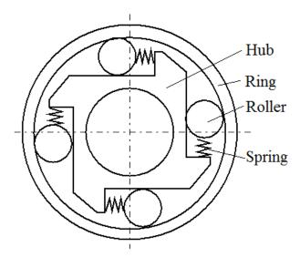
If locked, the clutch transmits torque from the hub to the ring. If unlocked, the clutch transmits no torque. The clutch does not have a state of being unlocked but engaged (transmitting torque). The relative angular velocity (slip),  $\omega$ , is the angular velocity of hub,  $\omega_H$ , relative to the velocity of the ring,  $\omega_R$ , that is,  $\omega = \omega_H - \omega_R$ .
