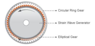
The internal meshing between the two gears causes the elliptical gear axis to spin counter to the elliptical strain wave generator.
