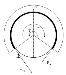
The braking torque as a function of the external brake actuation force that tightens the belt is
