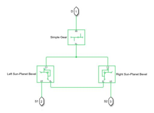
To increase the fidelity of the gear model, specify properties such as gear inertia, meshing losses, and viscous losses. By default, gear inertia and viscous losses are assumed to be negligible. The block enables you to specify the inertias of the gear carrier and internal planet gears. To model the inertias of the outer gears, connect Simscape Inertia blocks to ports  $\mathbf{D}$ ,  $\mathbf{S1}$ , and  $\mathbf{S2}$ .
