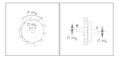
The cycloidal drive can operate in reverse mode, that is, with power flowing from the follower shaft to the base shaft. In reverse mode, torque transfer efficiencies are typically negligible. You can adjust the efficiency by changing the value of the **Efficiency from follower shaft to base shaft** parameter.
