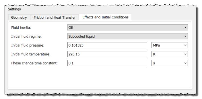
If you change the **Fluid Inertia** parameter from **Off** to **On**, the **Initial mass flow rate from port A to port B** parameter becomes visible. The table shows this dependency in rows 1, 2, and 7.
