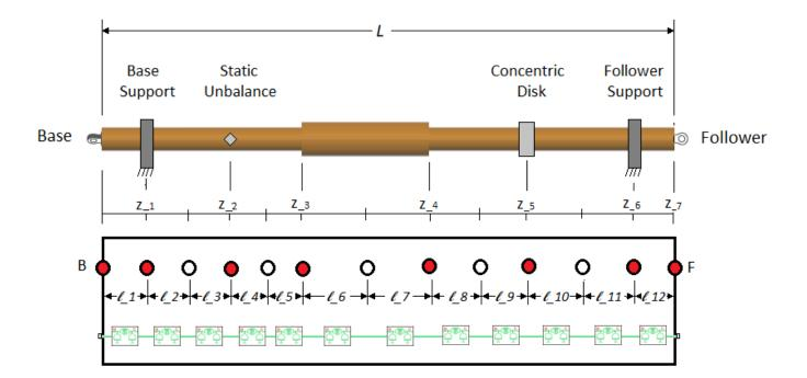
If  $N_{min}$  is large enough to yield a number of unfixed nodes that is greater than the number of fixed nodes, the block distributes more than one unfixed node between each set of neighboring fixed nodes.
