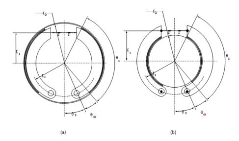
The model uses the long-shoe approximation. The equations for the friction torque that the leading and trailing shoes develop are:
