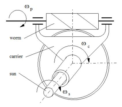
You specify a fixed gear ratio, which signifies the worm angular velocity divided by the sun gear angular velocity. You control the direction by setting the worm thread type to left-hand or right-hand. Rotation of the right-hand worm in the positive direction causes the sun gear to rotate in the positive direction. The positive directions of the sun gear and the carrier are the same.
