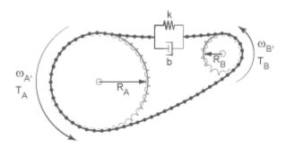
The chain tensile force is the net sum of the spring and damper forces. The spring force is the product of the tensile strain and the spring stiffness constant. This force is zero when the tensile strain is smaller than the chain slack. The damper force is the product of the tensile strain rate and the damping coefficient. Mathematically,
