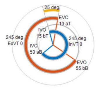
This plot shows a typical valve timing scenario where IVO occurs 15 degrees before TDC, and IVC occurs 50 degrees after BDC. EVO occurs at 55 degrees before BDC, and EVC occurs at 10 degrees after TDC. Note the 25 degrees of positive overlap where the intake valves open before the exhaust valves close. The table demonstrates the six valve overlap modes.
