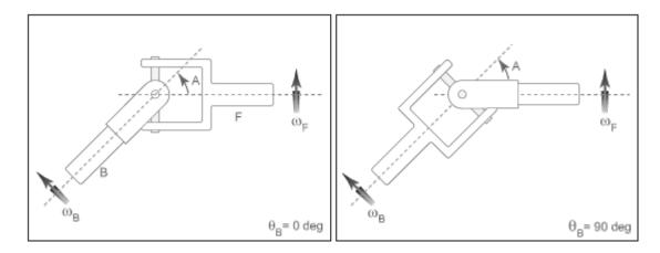
In the figure, the intersection angle is the angle between the two shafts about the pin of the base shaft. The absolute value of this angle must fall in the range  $0 \le A < Maximum intersection$  angle. The base shaft angle is the angle of the base shaft about its length axis. The base shaft angle is also the time-integral of the base shaft angular velocity,  $\omega_B$ .
