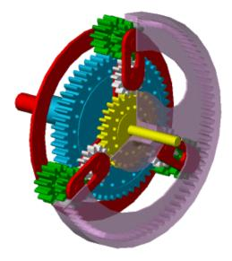
The block models the Ravigneaux gear as a structural component based on the Sun-Planet, Planet-Planet, and Ring-Planet Simscape Driveline blocks. The figure shows the equivalent block diagram of this structural component.
