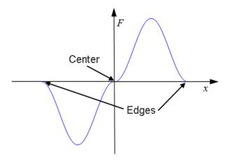
When you set **Parameterization** to By geometry, the block uses four regions to define the shear force. The figure displays these regions.
