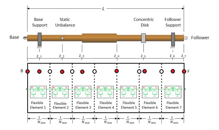
Note that the block did not add a node at  $z_4$  because a node was already added in the previous step of the algorithm. However, the node is now fixed because it represents a physical entity along the shaft length.
