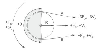
The sign convention is such that, when **Belt direction** is Ends move in opposite direction, a positive rotation in port S results in a negative translation for port A and a positive translation for port B.
