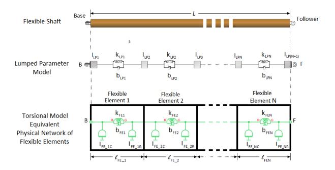
The block models the shaft as an equivalent physical network of N flexible elements. Each flexible element,  $FE_i$ , represents a short section of the driveshaft and contains:
