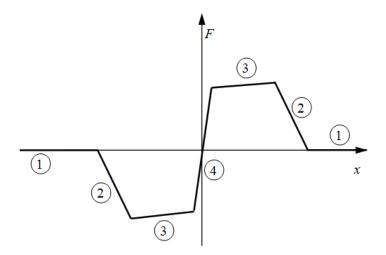
Because the ball is spherical and the notch is symmetric, the horizontal force versus displacement function is symmetric about the origin.
