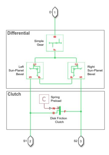
The ports of the Limited-Slip Differential block are associated with the driveshaft (port  $\mathbf{D}$ ) and the two driven shafts (ports  $\mathbf{S1}$  and  $\mathbf{S2}$ ), which connect the sun gears to the wheels.
