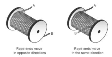
During normal operation, a driving torque causes the cylindrical drum to rotate about its axis of symmetry. The rotating drum transmits tensile force to the rope ends, which translate with respect to the drum centerline. The relative direction of translation between the two rope ends depends on the setting of the **Rope windup type** parameter. However, a positive drum rotation always corresponds to a positive translation at port **A**.
