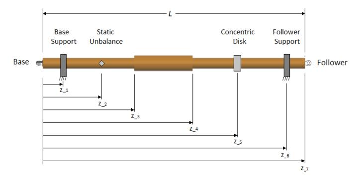
If model bending is on, the torsion model flexible element locations account for the locations of static unbalances and concentric rigid masses, so that the torsion flexible elements align with the bending flexible elements. During simulation, the torsion model is independent of any static unbalances or concentric rigid masses.
