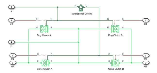
The model implements two Dog Clutch blocks, two Cone Clutch blocks, and one Translational Detent block. Refer to each block reference page for more information on the corresponding block function.
